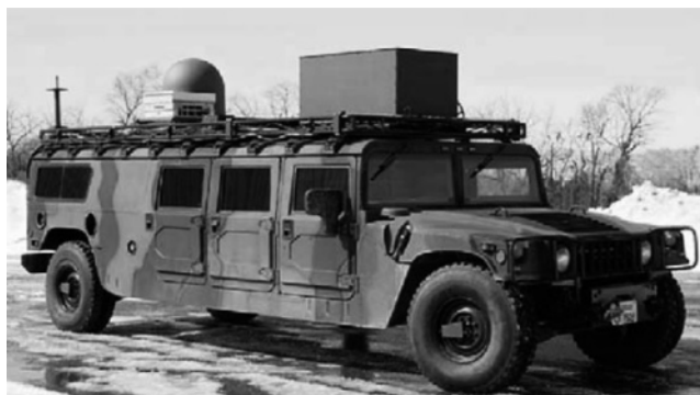
Figure 19. A command and control combat vehicle with a 2kW Idatech fuel cell APU mounted on the front portion of the roof. (Reprinted from ref 39, copyright 2004, with permission from Elsevier.)
