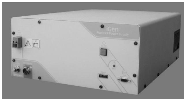
Figure 20. IdaTech's iGen Fuel Cell System generates 250 W at 12/24 VDC using a methanol/water mixture in a fully automated system about the size of two lunch boxes. (Copyright 2002–2006, Idatech, LLC, used by permission.)
