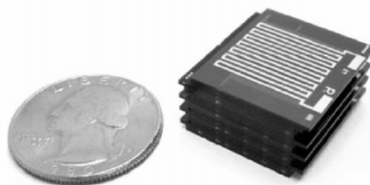
Figure 11. Casio-developed multilayered microreactor: (a) schematic cross-section of the reactor body indicating the various sections, and (b) picture of the device with a U.S. quarter for scale. (Reprinted from ref 195, copyright 2005, with permission from Elsevier.)
