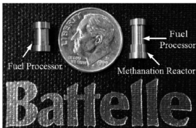
Figure 5. Sub-watt integrated methanol steam reformer developed at PNNL, without selective methanation (left) and with selective methanation (right). (Reprinted from ref 208, copyright 2004, with permission from Elsevier.)
